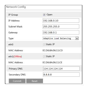
You will get a virtual IP address if the IP group is enabled. As to the access of the virtual IP address, the operation system of the server will judge and transfer the access to eth0 or eth1 automatically. For instance, if you disconnect the network cable of eth1 when testing "ping 192.168.0.10 –t", you will probably get a "Request Timeout" tip if you ping 192.168.0.10; and then you can probably ping it successfully after a few seconds.
